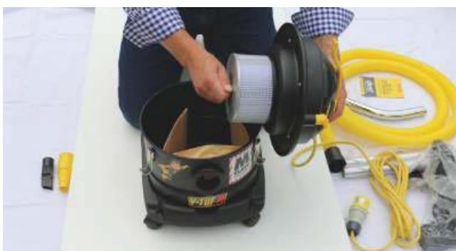
11 Ensure the filter retainer screw is tight
