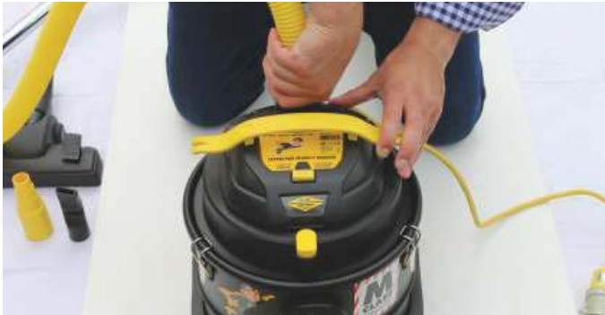
27 To use the blow feature, simply connect the hose to the exhaust port on top of the unit (as you would to the suction port)
