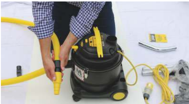
15 Fit power tool adaptor to extract dust from power tools
