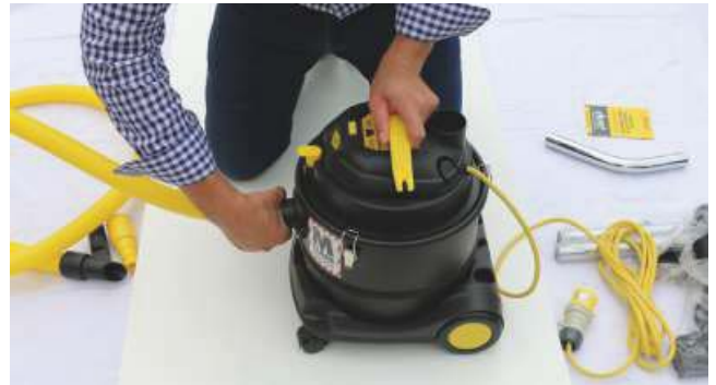
14 Turn clockwise to lock (gently pull to ensure it is locked)
